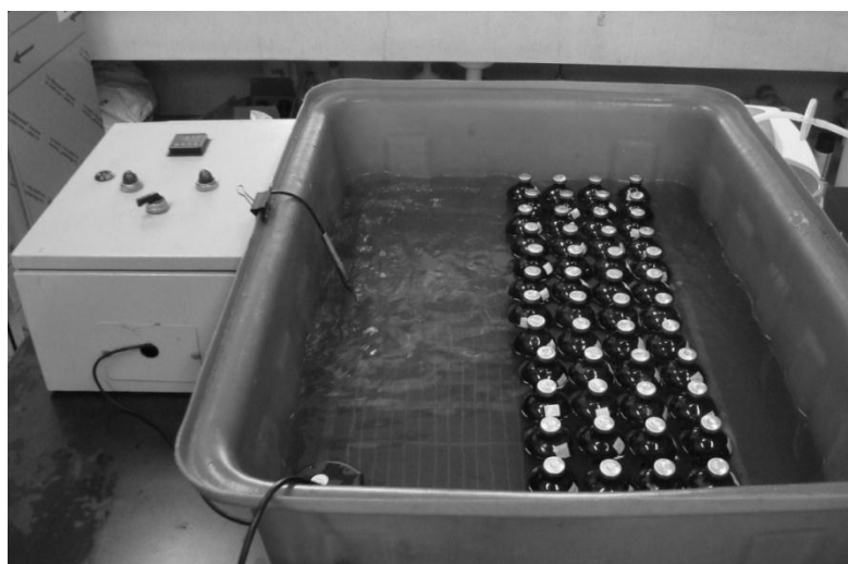
Fig 1. Bottles are placed in water - bath temperature controlled 38°C
