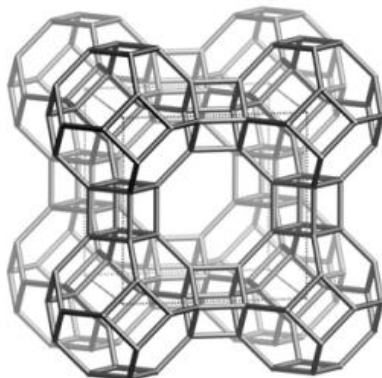
Fig 1. Structure of type-A zeolite [1]
